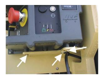
Remove the three bolts at the bottom of the ground control station.
